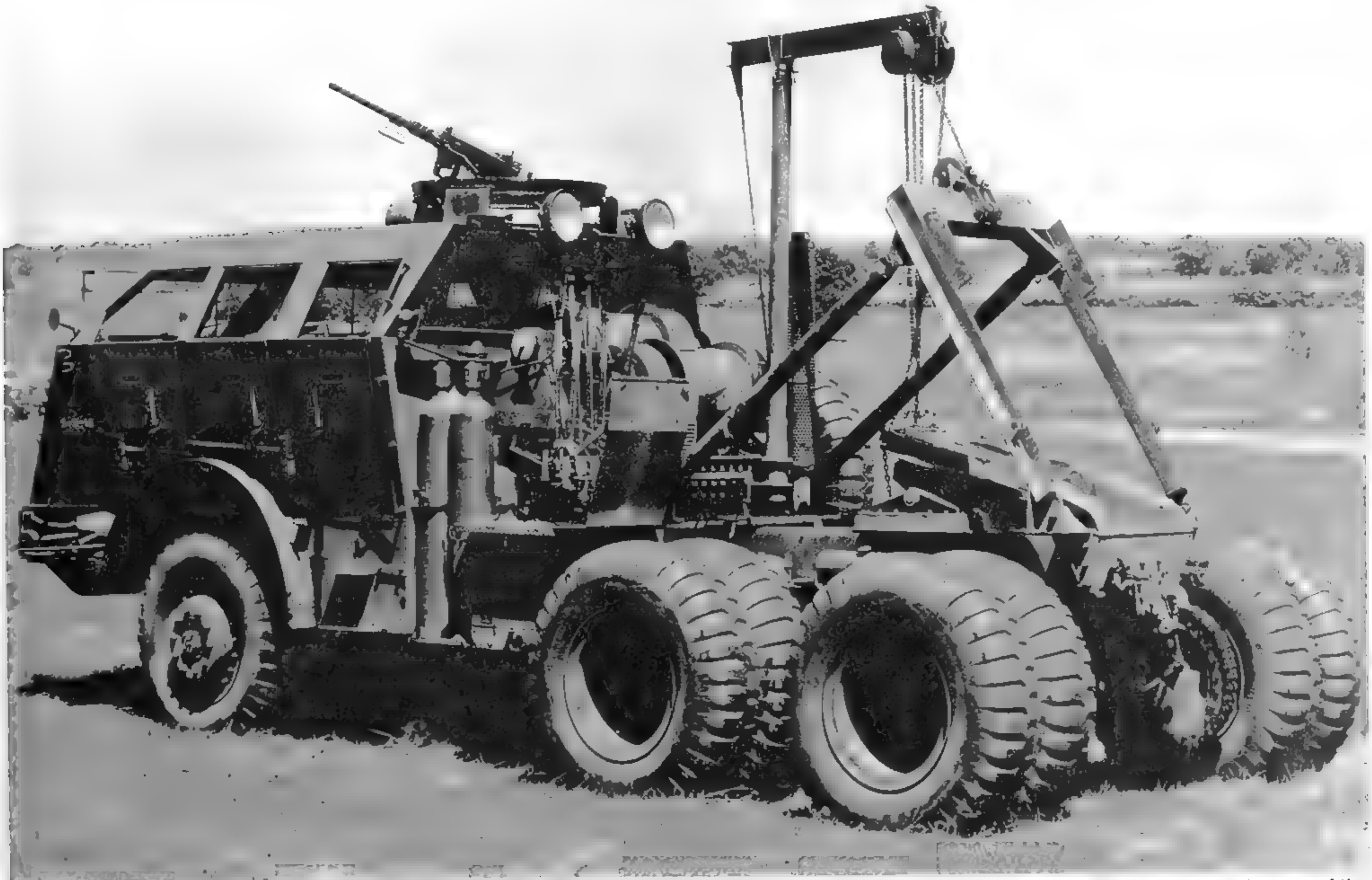
The M26 was provided with a large davit and chain hoist for use in repair operations and to handle the heavy spare tire. The A-frame at the rear of the truck could be set up in five different positions for different recovery operations. (U.S. Army photo)
